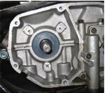
Disconnect the wires from the old dynamo. Pull all wires out of the engine housing.
