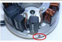
Have a look at the new stator. You will find on the circumference of its baseplate a small red marking. That to is an ignition marking.
