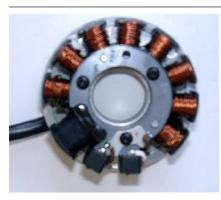
Put the stator coil back onto the plate, take care not the damage the wires. the stator has to snap in rather sharply. If it sets soft, you have probably squeezed a wire underneath!
