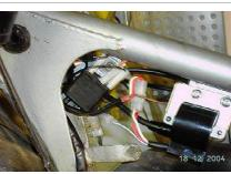
Fasten the electronic regulator on the frame.
