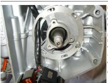
Unscrew the stator coil from the base plate and lift it a little away from it so that you can access the mounting holes. Take care not to damage the paint insulation of the coil.
